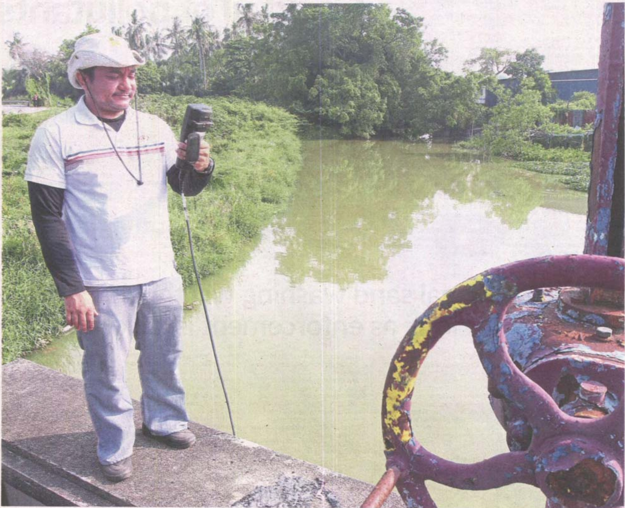
Extremely polluted: Water quality specialist Dr Zaki Zainudin checking the reading on an in-situ dissolved oxygen (DO) meter that measures level of pollution in rivers. The DO reading from Sungai Puloh in Klang is 0.22 mg/L. A healthy river will have a reading of between 7 and 8mg/L. — AZLINA ABDULLAH/The Star
